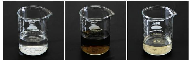
DI water (left) followed by addition of  $\text{FeCl}_3$  (Iron Chloride) and  $\text{Na}_2\text{S}$  (Sodium Sulfide) to afford in situ generation of FeS (Iron Sulfide) (middle) after a ScavSol AF 50 treatment to sequester the  $\text{Fe}^{3+}$  ions (right).
